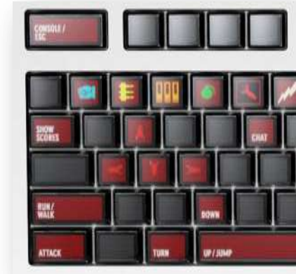
"Maximus" Keyboard Each key OLED display
